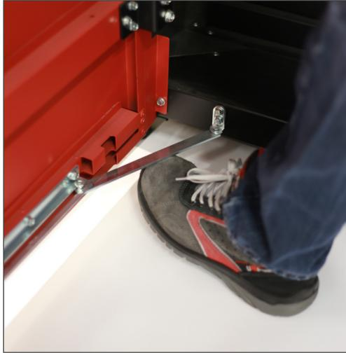
*Fig.1-10: Door lock Mechanism*
