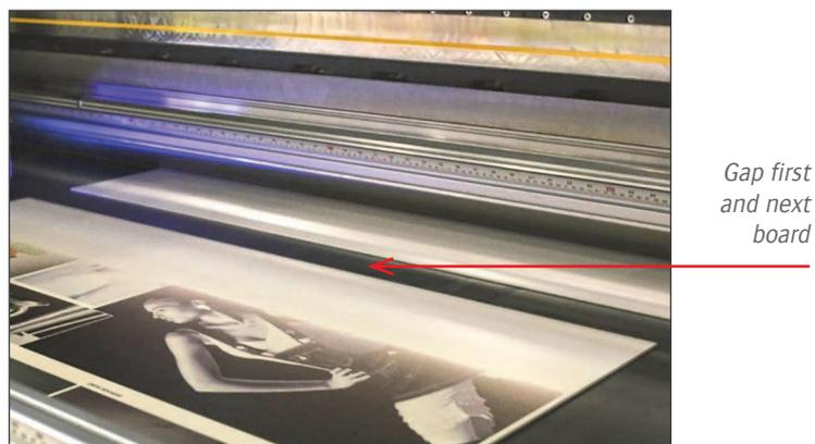
Fig.5-27: Board on Output Side - Manual Continuous Mode
