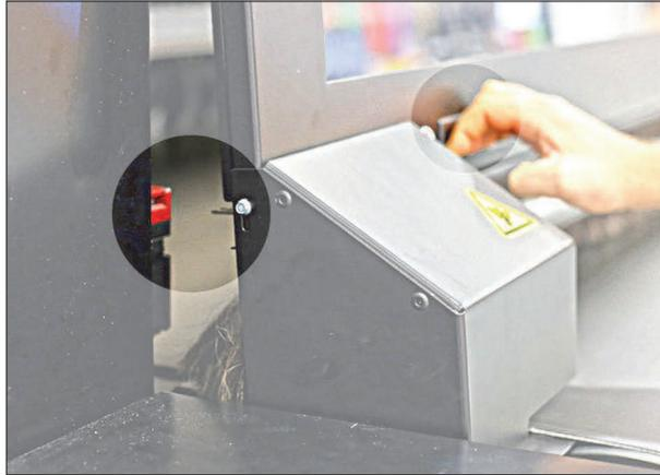
Fig.5-47: Door Interlock and Handle
