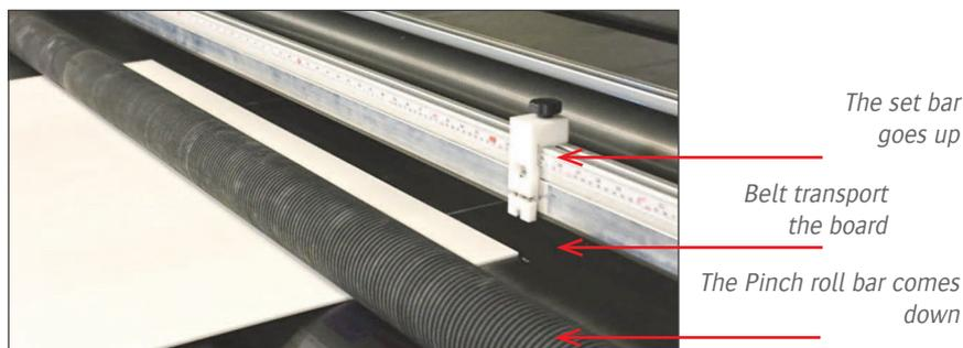
Fig.5-25: First Board Loaded - Manual Continuous Mode
