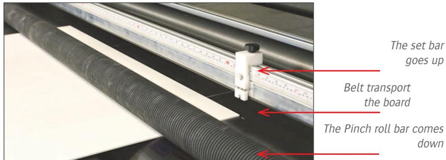
Fig.5-25: First Board Loaded - Manual Continuous Mode
